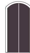
Porta a due ante ad arco a sesto ribassato Double leaf with lowered arch
