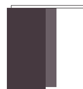
Porta scorrevole esterno muro composta Outside the wall sliding door with two overlapping single leaves
