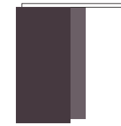
Porta scorrevole esterno muro composta Outside the wall sliding door with two overlapping double leaves
